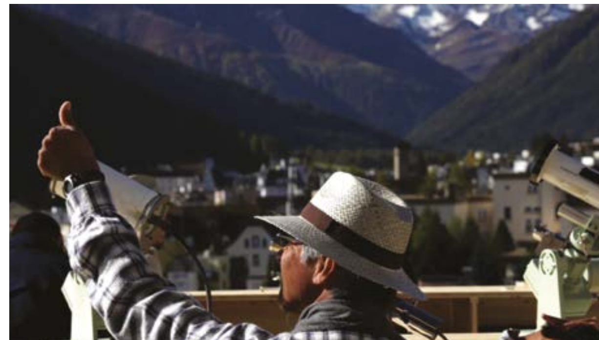
Figure 70. If one can cover the sun with the thumb, the atmosphere is clear and measurements will be good.
