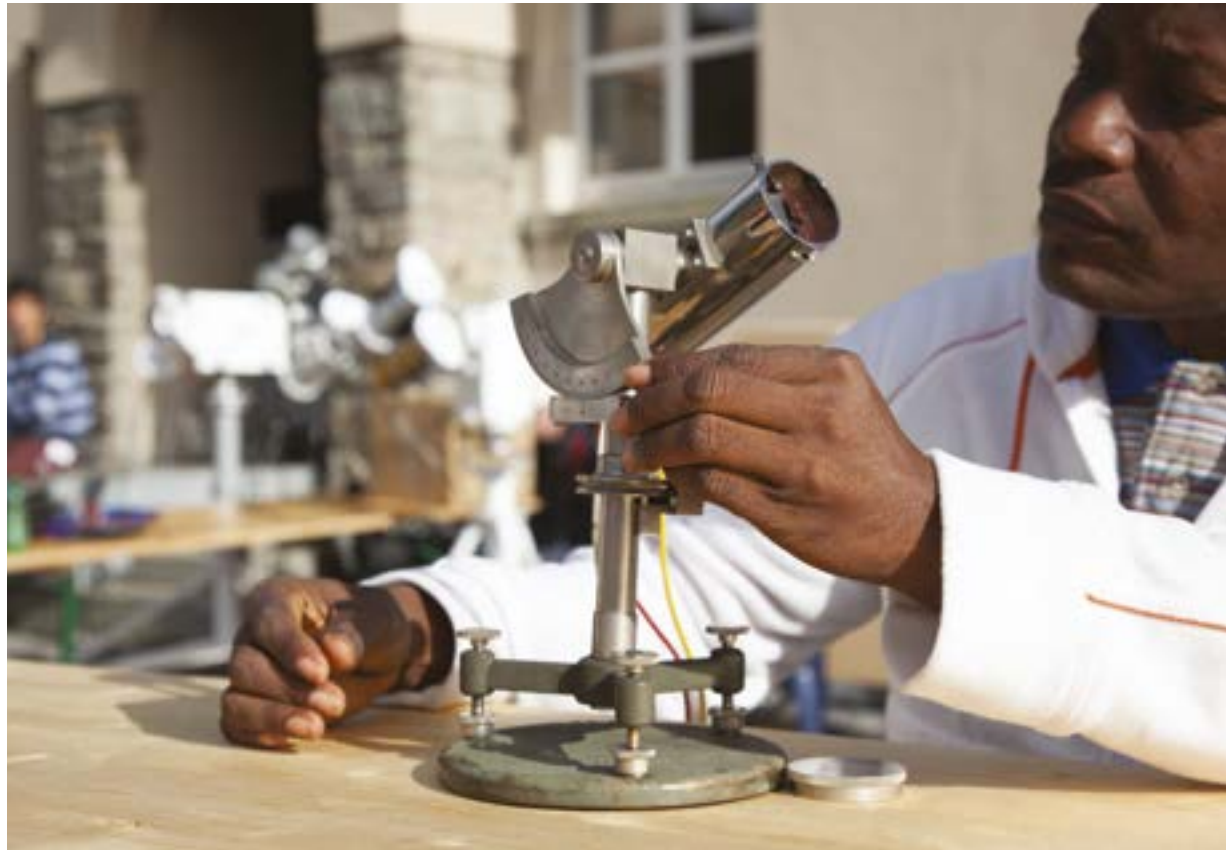
Figure 64. A Pyrheliometer is an instrument that reveals the difference between the energy level in a tube-like cavity when the sun shines directly into it and when it is closed.
